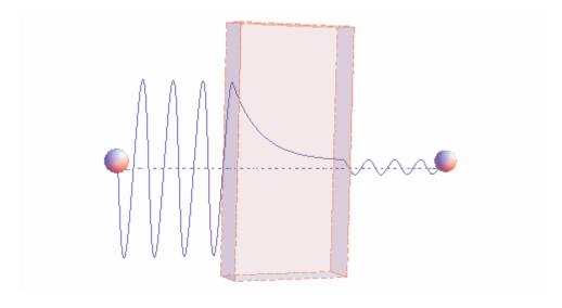
Schematic representation of quantum tunnelling through a barrier. The energy of the tunneled particle is the same, only the quantum amplitude (and hence the probability of the process) is decreased.
